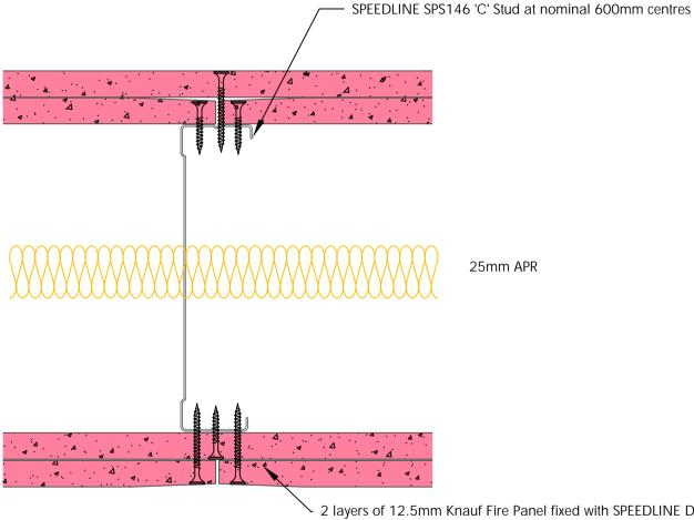
2 layers of 12.5mm Knauf Fire Panel fixed with SPEEDLINE Drywall Screws at 300mm centres (200mm centres at external angles). Ref to table for fixing length.
